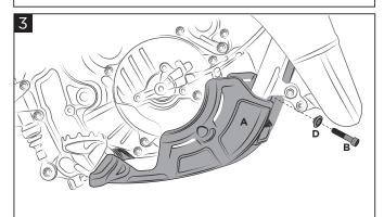
Secure the Skidplate (A) to the frame through the bolt (B) and the bushing (D).
