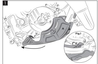
With force, push the skid plate (A) back towards the rear as indicated with the arrow. Make sure that the hook on the back of the skid plate is securely placed up and over the rear frame support
